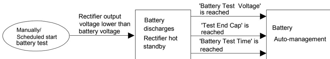
Figure 4-33 Schematic diagram of the test function
