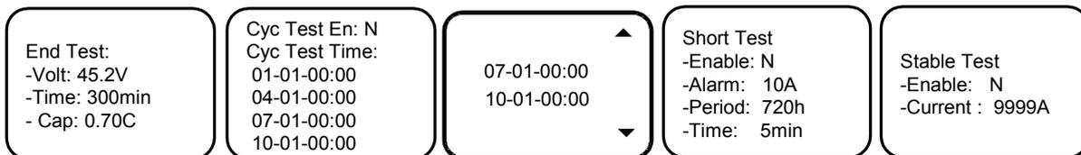
Figure 4-32 Battery test parameters screen
