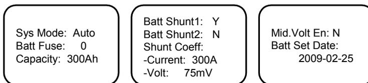
Figure 4-28 Battery basic parameter setting screen
