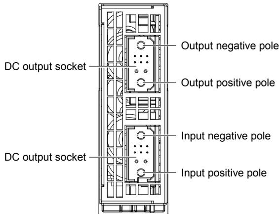
Figure 7 Rear panel of the solar module
