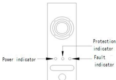
Figure 6 Front panel of the solar module
