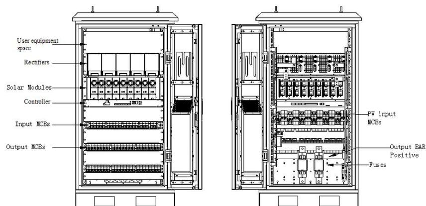
Figure 1-2 Structure diagram
